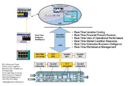
The historian server collects critical data from each DCS and other production layer systems. Most connections between the DCS and IT layer are through bi-directional communications. Process data moves from the DCS to the historian server and is then transmitted back to the DCS for management-level reports and dashboards.
