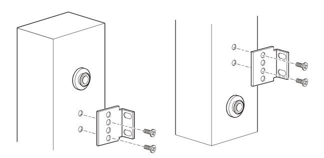
2. Install the PDU on a vertical mounting rail in your rack or enclosure.
