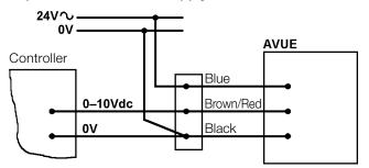
Up to 10 AVUE actuators can be connected in parallel. Ensure that the 24Vac supply is rated to operate the number of AVUEs connected to it.
