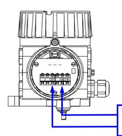
Analog output 4 to 20 mA System 2 wires Supply voltage DC 11 to 48V
