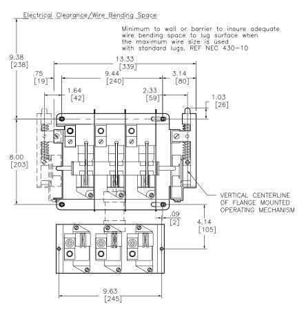
Distance from outside of flange to the circuit breaker mounting surface. 9.12 MIN, 19.25 MAX [232] **[489]** [232] 6.50 [165] 9.53 [242] 15.45 [393]
