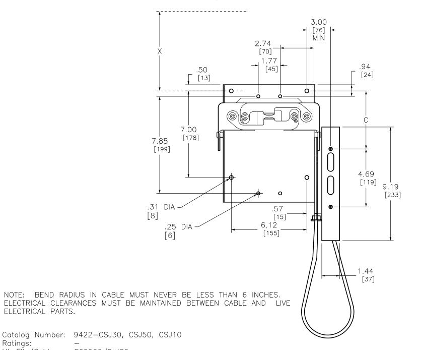
CABLE MECHANISMS FOR USE WITH CLASS 9422 TYPE NSJ 3 POLE CIRCUIT BREAKER. MAXIMUM DISTANCE FROM TOP RIGHT MOUNTING HOLE MAXIMUM CABLE TO UPPER MOUNTING HOLE TYPE BOX LENGTH FOR HANDLE OPERATOR (DIM C) DEPTH MINIMUM C MAXIMUM C CSJ30 36" 24" 3.75" CSJ50 36" 24" 60" 3.75" 36" 3.75" 5 FEET CSJ10 120"
