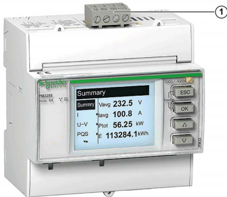
1 Modbus SL RS-485 2-wire port
