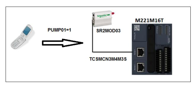
For example, you may send an SMS message to the GSM modem containing the command PUMP01=0, as represented in the graphic above.
