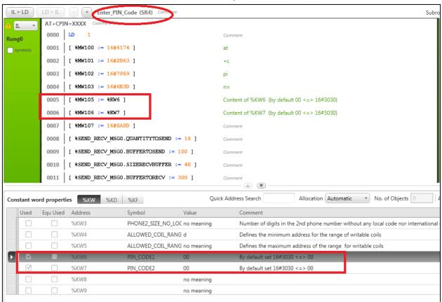
Setting the memory bit %M59 to 1 sends the PIN code to the modem.
