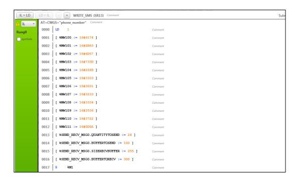
Modify the number, retaining all other characters including the quotation marks. Then, adjust the number of characters to be sent to the modem, contained in <code>%SEND\_RECV\_MSGO.QUANTITYTOSEND</code> (set to 24 in the template example).
