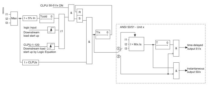
Action of the CLPU 50/51 function on set point Is of ANSI 50/51 protection unit x during time delay T/x depends on the Global action CLPU 50/51 setting:
