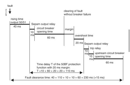
The time delay for the 50BF function is the sum of the following times:
