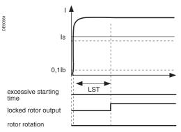
Case of starting locked rotor.
