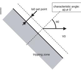
Tripping characteristic of protection function 67N type 1  $(\theta 0 \neq 0^{\circ})$ .
