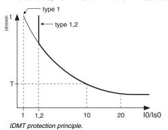
The Is0 setting is the vertical asymptote of the curve, and T is the operation time delay for 10 Is0.
