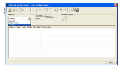
Configuration windows for the communication network, according to the type of link: serial link, modem link (STN) or Ethernet link (TCP).
