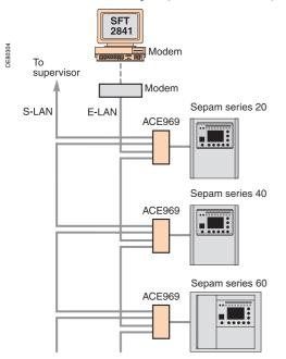
SFT2841 connected to a Sepam network
