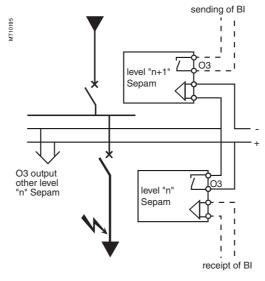
When a fault occurs in a radial network, the fault current flows through the circuit between the source and the location of the fault:
