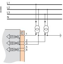
When a ground fault occurs on a TT or IT network, the neutral potential is affected: the neutral cannot act as a reference for the VTs, phase-to-phase voltages must be used on both phases.
