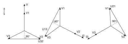
Three-phase function: polarization currents and voltages.
