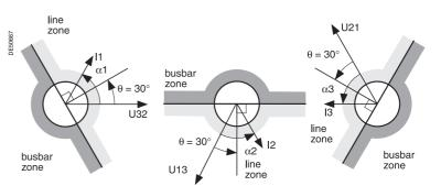
Fault tripping in line zone with  $\theta = 30^{\circ}$ .
