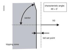
Tripping characteristic of protection function 67N type 1  $(\theta 0 = 0^{\circ})$ .
