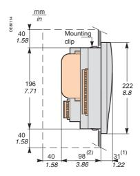
Sepam with advanced UMI and MES114, flush-mounted in front panel.
