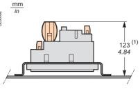
Sepam with basic UMI and MES114, mounted with AMT840 plate. Mounting plate thickness: 2 mm (0.079 in).
