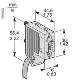
Male 9-pin sub-D connector supplied with the ACE919.
