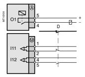
Wiring for undervoltage trip unit.
