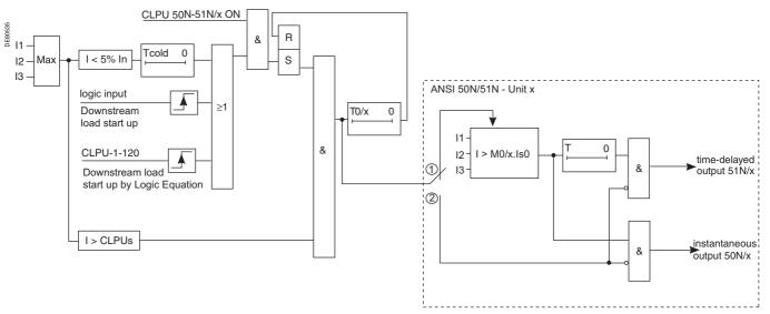
Action of the CLPU 50N/51N function on set point Is0 of ANSI 50N/51N protection unit x during time delay T0/x depends on the Global action CLPU 50N/51N setting:
