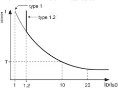
The Is setting is the vertical asymptote of the curve, and T is the operation time delay
