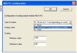
Analog output module (MSA141) setting window.
