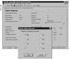
"Sepam diagnosis and output relay test" screen.
