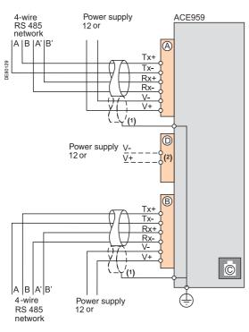
(1) Distributed power supply with separate wiring or included in the shielded cable (3 pairs).(2) Terminal block for connection of the distributed power
