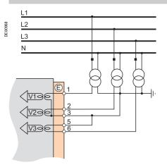
When a ground fault occurs on a TN-S or TN-C network, the neutral potential is not affected: the neutral can act as a reference for the VTs.
