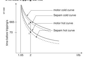
For an overload of 2\*lb, the value t/T1 = 0.0339(2) is obtained.
