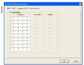
SFT2841: IP filtering configuration.
