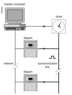
Architecture for "external synchronization" via a logic input.
