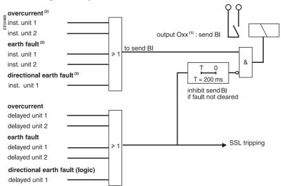
The protection units must be configured to trip the circuit breaker in order to be taken into account in logic discrimination.
