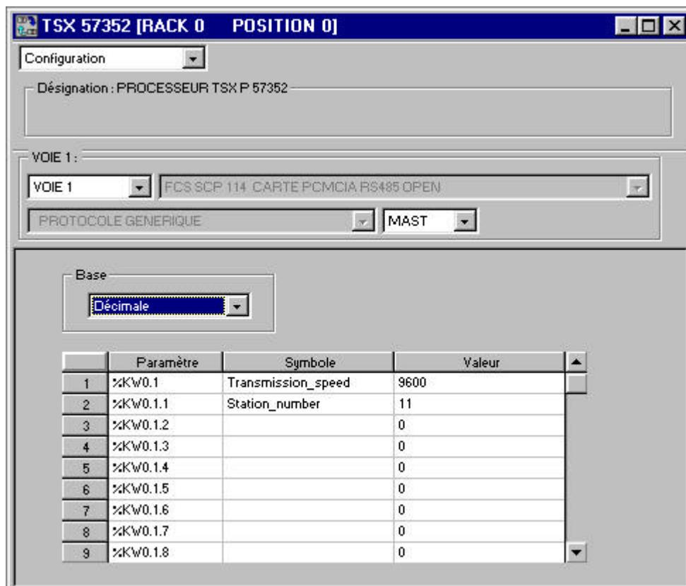
With Symax protocol, the user must configure 2 words %KW0.1.0 and %KW0.1.1. The different values for these parameters are :
