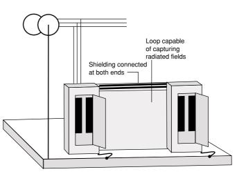
Note that overvoltages may be caused by separate earth electrodes for which the potentials vary differently.
