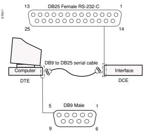
Some terminals and computers may have a DB9 type RS-232-C serial connector. In the figure above, the RS-232-C serial connection uses a DB9 to DB25 cable.
