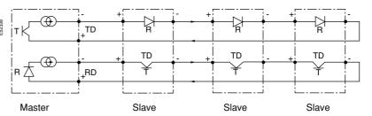
■ Transmitters for slave stations can be connected in parallel with the receivers of the master station. In this case the resting state of the line is 0 mA:
