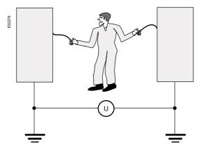
To ensure trouble-free operation of equipment and the safety of persons, all exposed conductive parts must be interconnected and earthed to ensure equipotentiality.
