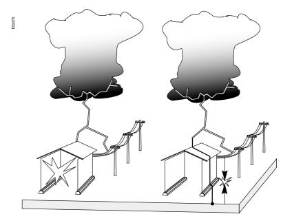
**Definition:** An exposed conductive part is an accessible metal part that is isolated with respect to the live parts of the equipment but which may accidentally become live.
