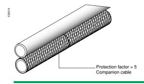
A raceway increases protection by a factor of approximately 50 between 1 MHz and 100 MHz.
