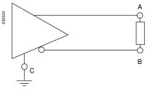
Line "A" on the transmitter is negative with respect to line "B" for a binary "1" (OFF). Line "A" on the transmitter is positive with respect to line "B" for a binary "0" (ON).
