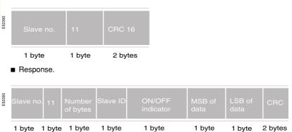
**Note:** The number of bytes, slave ID and data available depend on the type of slave. For the ON/OFF indicator: FF = ON & 00 = OFF.
