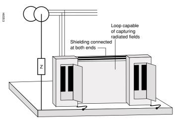
An initial insulation fault can lead to a phase-to-phase voltage between a phase conductor and the equipment ground.
