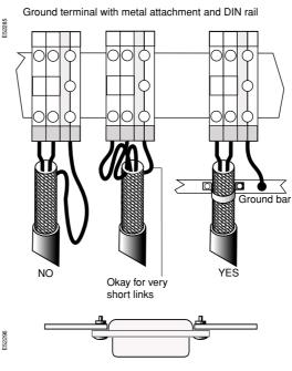
If a connector is used, it must provide a 360° electrical continuity between the cable shielding and the equipment ground.
