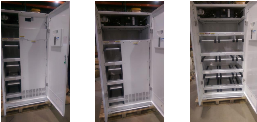
Figure 33 : Removal of dead front
