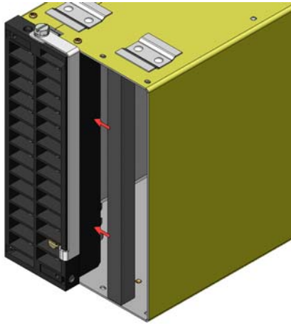
Figure 11: In direction of arrows attach adhesive side of rubber sealing strip to side wall of terminal block.
