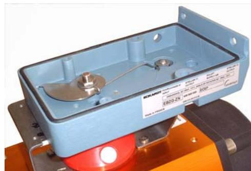
d) Mount cam **24** in accordance with the direction of rotation of the actuator.
