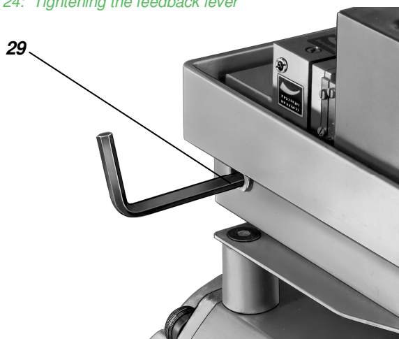
Fig. 24: Tightening the feedback lever
