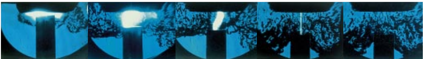
Electric arc in a self-expansion breaking chamber.
