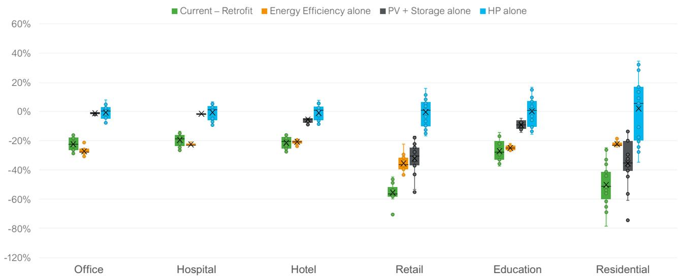
Figure 46 – Energy spend savings per segment, and per key contribution, new constructions
