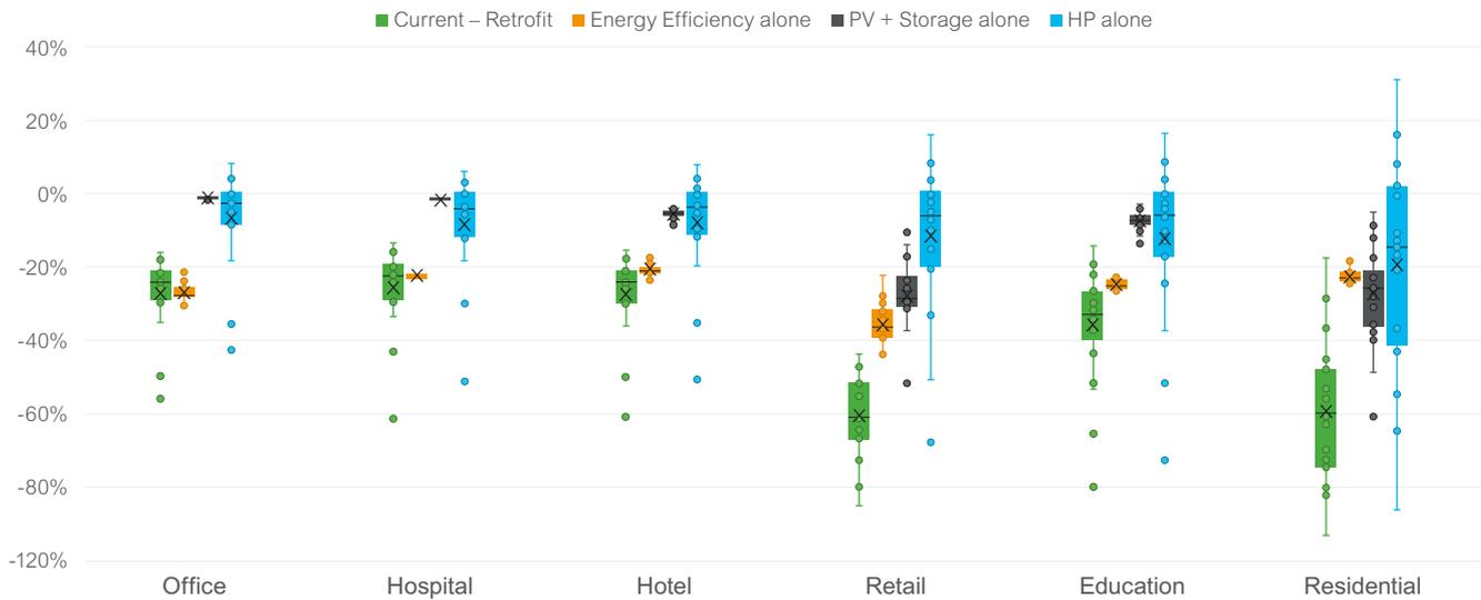
Figure 45 – CO<sub>2</sub> abatement per segment, and per key contribution, new constructions
