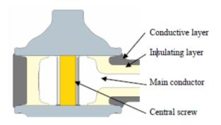
All the external surfaces of the installed interconnector system are screened and connected to the earth. The electrical field is totally included and fixed in the insulating layer without affecting the surface of the interconnector, avoiding any superficial electrical aging.
