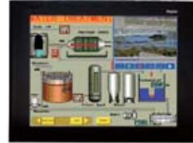
Back-lit color TFT LCD (1024 x 768 pixels)
