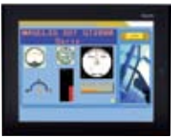
Back-lit color STN LCD or TFT LCD (640 x 480 pixels)
