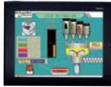
Back-lit color TFT LCD (800 x 600 pixels)
