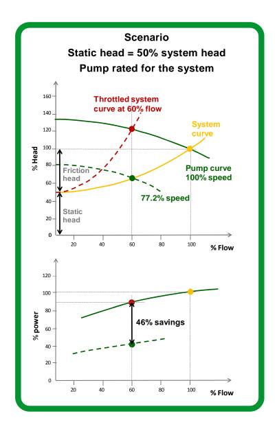
The example in **Figure 1** compares two installations (one with a variable speed drive one with a fixed drive throttled system) in which static heads (height difference between the source and the end use) are different.
