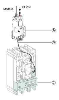
A IFM Modbus-SL interface for one circuit breaker
