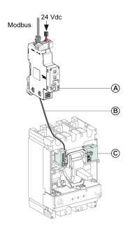
A IFM Modbus-SL interface for one circuit breaker
