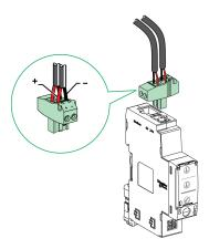
It is recommended to use an UL listed/UL recognized limited voltage/limited current or a class 2 power supply with a 24 Vdc, 3 A maximum.
