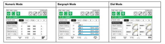
To read the voltage bar graph correctly, you must set up the primary nominal voltage of the circuit breaker.
