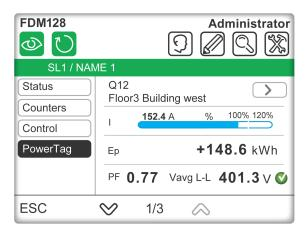
The below figure shows the PowerTag screen of Smartlink SI D, PowerTag Link HD, and EcoStruxure Panel Server gateway.
