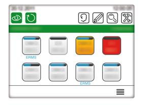
In the icon mode, the device with its ERMS mode engaged displays a blue ERMS message below the device icon.
