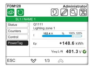
The following figure shows the PowerTag screen of Smartlink SI D and EcoStruxure Panel Server gateway.
