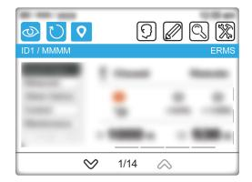
In the **Device view**, the device with its ERMS mode engaged displays an ERMS message in the title bar.
