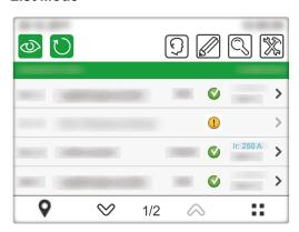
In the list mode, the device with its ERMS mode engaged displays the Ir settings in blue.
