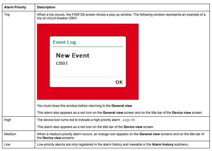
**NOTE:** The circuit breaker alarms configured using EcoStruxure Power Commission software are only registered in the alarm history and viewable in the Alarm history submenu. For information about configuring alarms using EcoStruxure Power Commission software, refer to the circuit breaker documentation.
