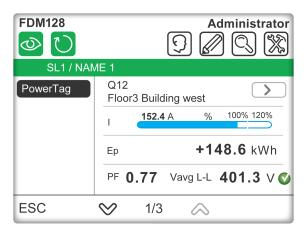
The following information is displayed in the submenu of PowerTag M250/M630 energy sensors:
