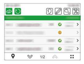
In the list mode, four devices are displayed per screen, one per line.
