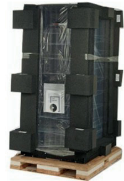
Completed rack on shock pallet ready for install
