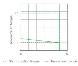
Its nominal torque is 5.2 Nm at 3,000 rpm, which produces 1.6 kW.
