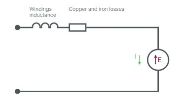
E is an image of the electromotive force of the machine, which depends on flux created by the magnets and the number of revolutions  $\omega$ .
