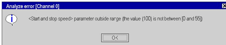
You must access the adjustment screen, correct the invalid parameter, then confirm.
