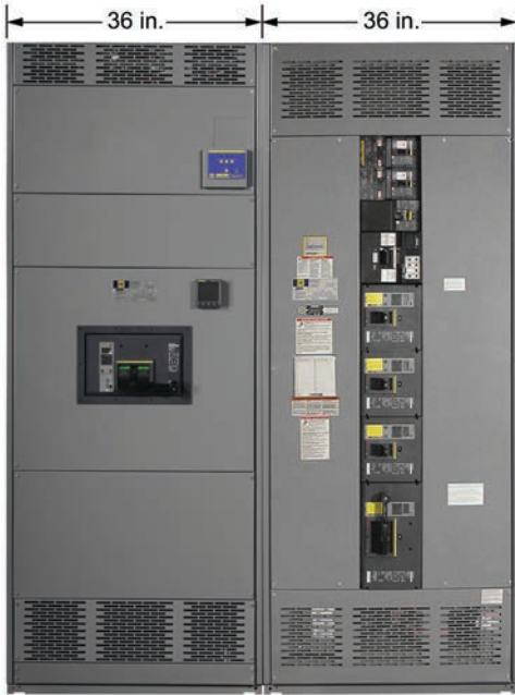
Shown is 2000 A, QED-2 Switchboard with 63 in. of Branch Circuit Breaker Mounting Height Available
